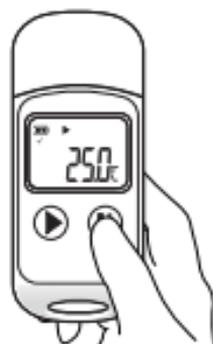
Press and hold the right key for 5 seconds to stop recording ③
