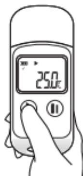
Press and hold the left key for 5 seconds to start recording ②
