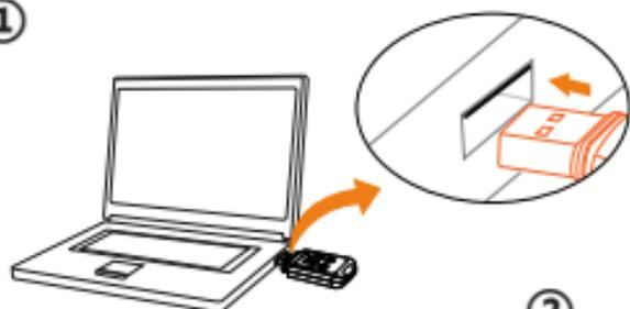
Connect the data logger to a computer to set configuration parameters ①
