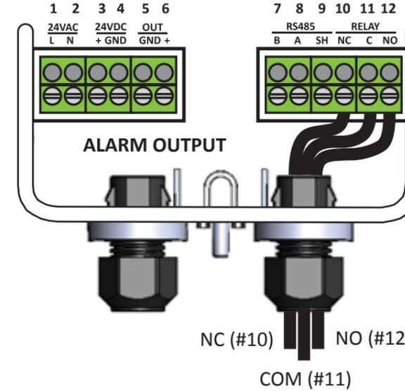
**NOTE:** After wiring is completed, carefully re-assemble the enclosure. After installation is complete, be sure to refer to the User Manual (part number 6490-9000) at [www.MyBacharach.com](http://www.MyBacharach.com) for additional instruction for proper operation.
