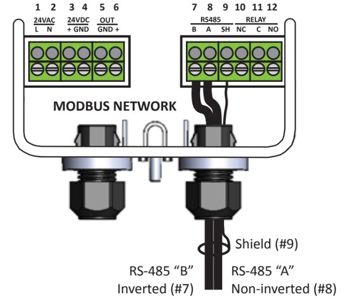
**IMPORTANT:** For Modbus network communications wiring, use only 18-24 AWG shielded twisted pair wire with 120 ohm characteristic impedance.
