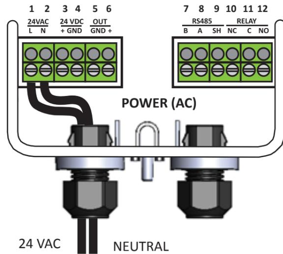
**WARNING:** The MGS-250 must be powered by either:
