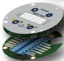
Processor Board (Middle Layer) with Keyed Ribbon Cable
