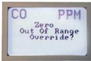
To override, move the second IDLE jumper from its rest position to the OVER / DESC / TEST position. If the jumper is not moved to the OVER position within 30 seconds, the calibration will be cancelled and the LPT-A will return to normal mode. After using the OVER / DESC / TEST position, the second IDLE jumper should be returned to its rest position.
