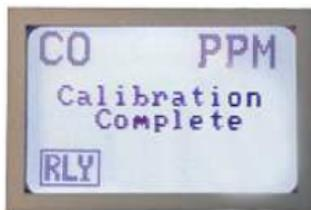
Return the jumpers back to the IDLE positions. Calibration is complete.
