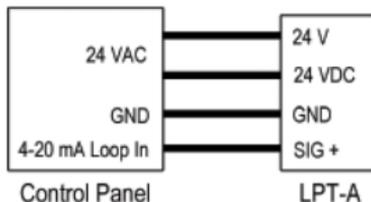
If the installer is powering the LPT-A with three wire 24 VDC or ground referenced AC, the “positive” wire should be connected to terminal “two” (AC / DC) and the negative wire should be connected to terminal “three” (GND). The “signal” (4 - 20 mA or 0 - 10 volt) wire is always connected to terminal “four”.
