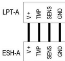
**The maximum length of wire between the ESH-A Remote Sensor and the transmitter should not exceed 200 ft (61 m).**
