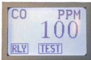
After 5 minutes (or when the jumper is removed from the OVER / DESC / TEST position), the unit will return to normal operation.
