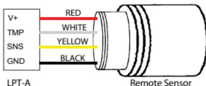
**The maximum length of wire between the ESH Remote Sensor (dongle style) and the transmitter should not exceed 50 ft (15 m).**
