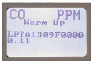
The warm up period is approximately 3 minutes (some gases, like Chlorine, may take a little longer). After the warm up period the device may exhibit gas alarm conditions if the sensor has not completely stabilized during the warm up period. This is normal and the length of time the gas alarm exists is dependent upon the length of time since the unit was last powered up and the state of the environment it is installed in.
