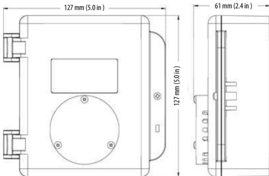
Above dimensions are shown with optional splash guard. Without splash guard, thickness is 53.34 mm (2.1 in). The area required for enclosure door to be open 90 degrees is 178 mm (7 in) or 254 mm (10 in) for fully open. With the splash guard, the enclosure has an IP54 rating.
