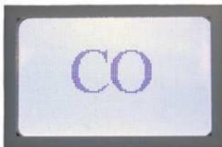
The display will be backlit but will only show the name of the gas (it will not show the gas readings) and any abnormal conditions, e.g. fault, etc.
