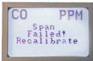
If the calculated sensitivity of the sensor is out of range the display will show 'SPAN FAILED!'
