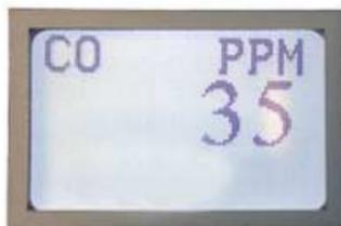
The display will be backlit and show the gas formula, the units and the current gas level. This is the factory default position.
