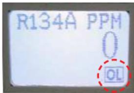
**NOTE:** If the voltage output is chosen, the open loop indicator on the circuit board will always be on. Refer to Section 4.2 *Interior System Layout* to find where the Open Loop LED is located.
