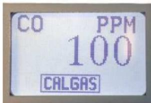
While adjusting the calibration gas value a corresponding voltage will be signaled on the test points TP-1 and TP-2. For example: a common calibration gas for CO is 100 ppm, which is half the range, so 2 volts at the test points indicates 100 ppm.
