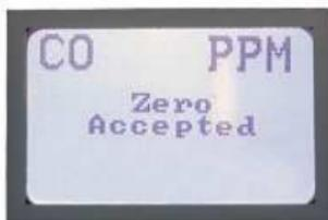
If the new zero value is all that is required, move the jumper back to the IDLE position and the full calibration procedure will be cancelled. A zero shift calibration is only done when the LPT-A is being installed for the first time. The reason for a zero shift calibration is to compensate for the new environment in which the LPT-A is being installed. To continue with the calibration procedure to Step 4.
