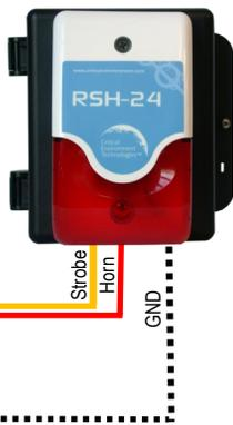
AS SHOWN, STROBE & HORN OPERATE TOGETHER.
