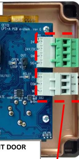
RELAY CONTROL WIRING TERMINAL.
