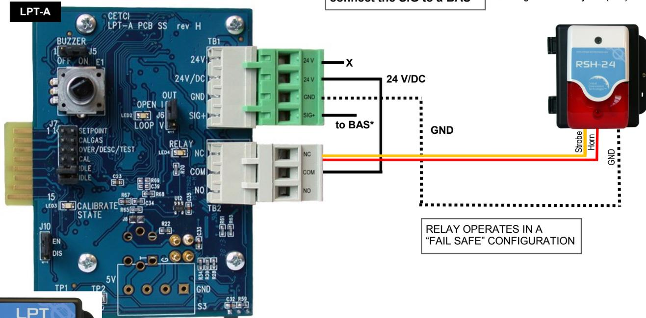
AS SHOWN, STROBE & HORN OPERATE TOGETHER.
