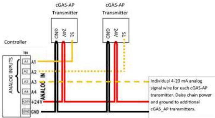
If the cGas Detector is being connected to a BAS, DDC or other control panel then either a 24 VDC power supply or 24 VAC Class 2 or better transformer need to be used.
