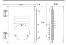
Note: Drawings above are shown with an optional splash guard. Without splash guard, thickness of unit is 2.1" (53 mm).
