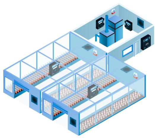
C3H8-100 remote sensor with an internal propane sensor should be used, mounted 6 inches off the finished floor, close to the pipes supplying the gas to the furnace. If the furnace uses natural gas, an ESH-A-CCH4-100 remote sensor with an internal methane sensor should be used instead, mounted 6 inches from the ceiling above the pipes supplying the gas. Inside the room should be an audible/visual alarm device such as the RSH-24V-R Remote Strobe/Horn.
