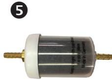
Flowing dry gas over solid state sensors can result in a negative reaction and inaccurate readings. Use the humidification chamber to increase the humidity and recreate a real-world environment for the sensor. Wet the sponge with water and gently squeeze out the excess. It should be quite damp before reinserting it into the humidification chamber. Remember to remove and dry out the sponge after use.
