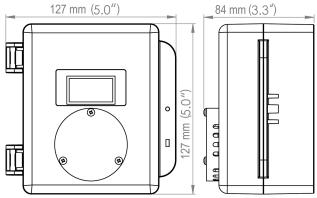
Above dimensions are shown with optional splash guard. Without splash guard, thickness is 71 mm / 2.8 in. The area required for enclosure door to be open 90 degrees is 178 mm / 7.0 in or 254 mm / 10.0 in for fully open. With the optional splash guard installed, the enclosure is IP54 rated.
