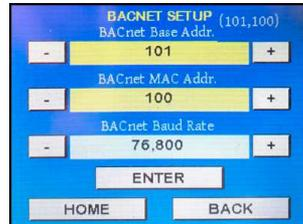
**BACnet Base Addr.:** Use the + and - buttons to increase or decrease the number until the correct BACnet base address is displayed, or press the yellow field and use the keypad to enter the number. The FCS factory default base address is 270. Press ENTER to save.
