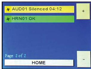
When the preconfigured silenced amount of time (OFF Delay) has passed, the strobe/horn and buzzer will sound and the Silence? screen will appear again. The silence interval is specific to each audible relay. The OFF Delay for that relay sets the silence duration.
