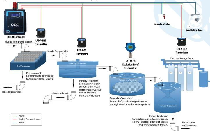
The treatment of waste water involves a combination of physical, chemical and biological processes that create several toxic and combustible gases. Some areas are enclosed spaces where gases can build up and deplete oxygen levels. In these areas, workers should be equipped with personal gas monitors to ensure the air is safe to breathe. Other areas are open and a fixed gas detection system is appropriate because it will provide continuous monitoring of the gases to ensure the area is safe.
