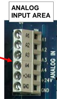
A1 TO A4 ARE INDIVIDUAL 4-20 mA SIGNAL WIRE CONNECTIONS FOR EACH TRANSMITTERS
