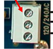
INSTALLER SUPPLIED LINE VOLTAGE (90-240 VAC, 50-60 HZ)
