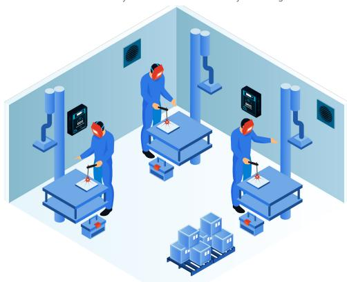
The DCC, with two internal sensors, one Carbon Monoxide (CO) and one Nitrogen Dioxide (NO<sub>2</sub>), should be mounted close to the welding work stations, in the "breathing zone" which is 1.2 to 1.8 meters (4 to 6 feet) from the floor. This is the height at which most humans breathe and the height at which these gases pool. In poorly ventilated areas, gases can accumulate and displace the oxygen causing an oxygen-deficient environment.
