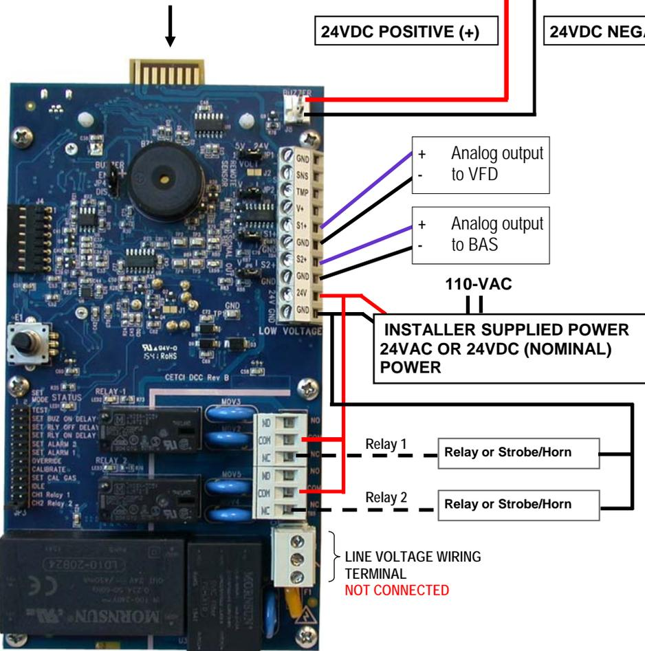
RELAY 1 IS COMMONLY CONFIGURED FOR LOW ALARM TRIGGERING OF A DEVICE.
