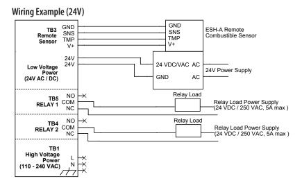
A class 2 or better transformer must be used. The stated max current draw of the SCC in this mode is 0.5 A.
