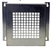
The metal protective guard is made of heavy duty metal and helps to protect against abrasive damage, theft or vandalism to the transmitter. It is made from 16-gauge galvanized steel and has ½" (13 mm) square openings in the front to allow gas and air to flow through to the sensor. With only four slotted mounting holes, installation and removal for gas detector servicing is easy.
