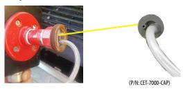
**NOTE:** Ammonia is a reactive gas and can adhere to surfaces which can reduce the amount of gas that reaches the sensor. When calibrating an ammonia sensor use a length of tubing no longer than 0.6 to 1 m / 2 to 3 ft. If a longer length is necessary, use Teflon lined tubing to ensure the correct concentration of gas reaches the sensor.
