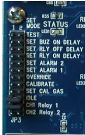
To start a configuration, place one jumper on the channel / relay select position CH1 Relay1 and place the other jumper on the function position you want to configure:
