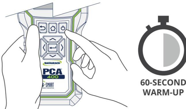
**IMPORTANT:** Perform power up and initialization in fresh air to ensure proper calibration.
