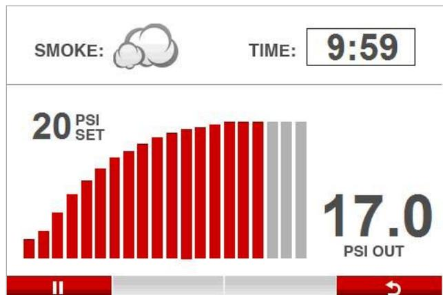
4. The screen displays the set pressure as well as the current output pressure. The test will automatically stop after 10 minutes.
