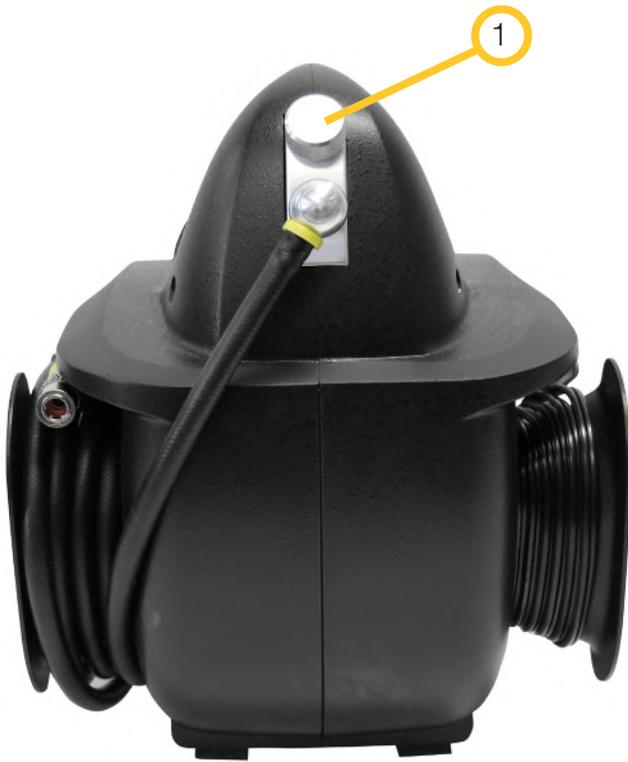
1. COOL SMOKE FLUID DIPSTICK: To check the fluid level insert dipstick until threads touch then remove and read.
