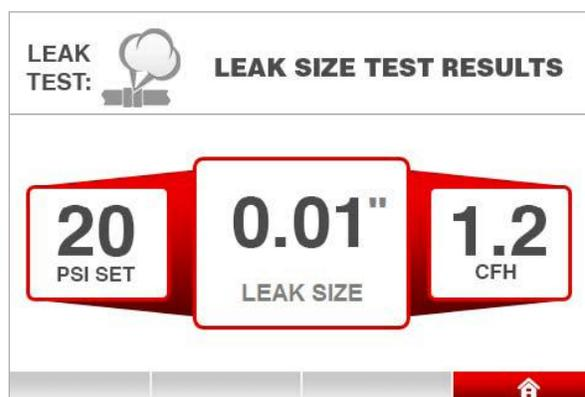
5. Results - When the output pressure stabilizes at the set pressure, the leak size results page will display the leak size and resulting flow rate from the test.
