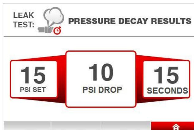
3. Results: When the pressure decay test is complete the results will be displayed. These results can be compared with the manufacturer’s specifications.
