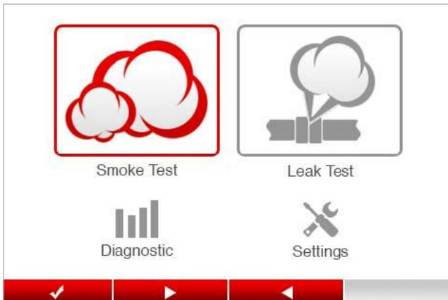
1. Select smoke test by pressing “select” (
