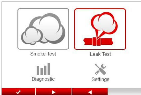
1. Select leak test by pressing "select" (
