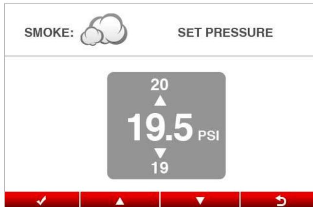
2. Set the test pressure by using the scroll buttons (
