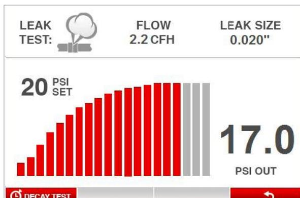
4. The machine will fill the system with pressurized smoke until the set pressure is reached.
