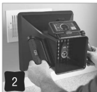
Capture Airflow Readings
