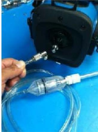
The Bar Hole Probe has two filters, the Hydrophobic Filter (102277-0) and the Particulate Filter (102276-0), located in the Bar Hole Probe handle. Unscrew probe handle and ensure that both filters are clean and dry. Replace if necessary.
