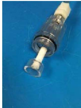
Put the Bar Hole Probe handle back together, making sure handle is screwed tightly together and O-ring makes a tight seal so no leaks will occur during survey. Also ensure that the sampling holes at the end of the Bar Hole Probe are not blocked or plugged. The probe is now ready for use.
