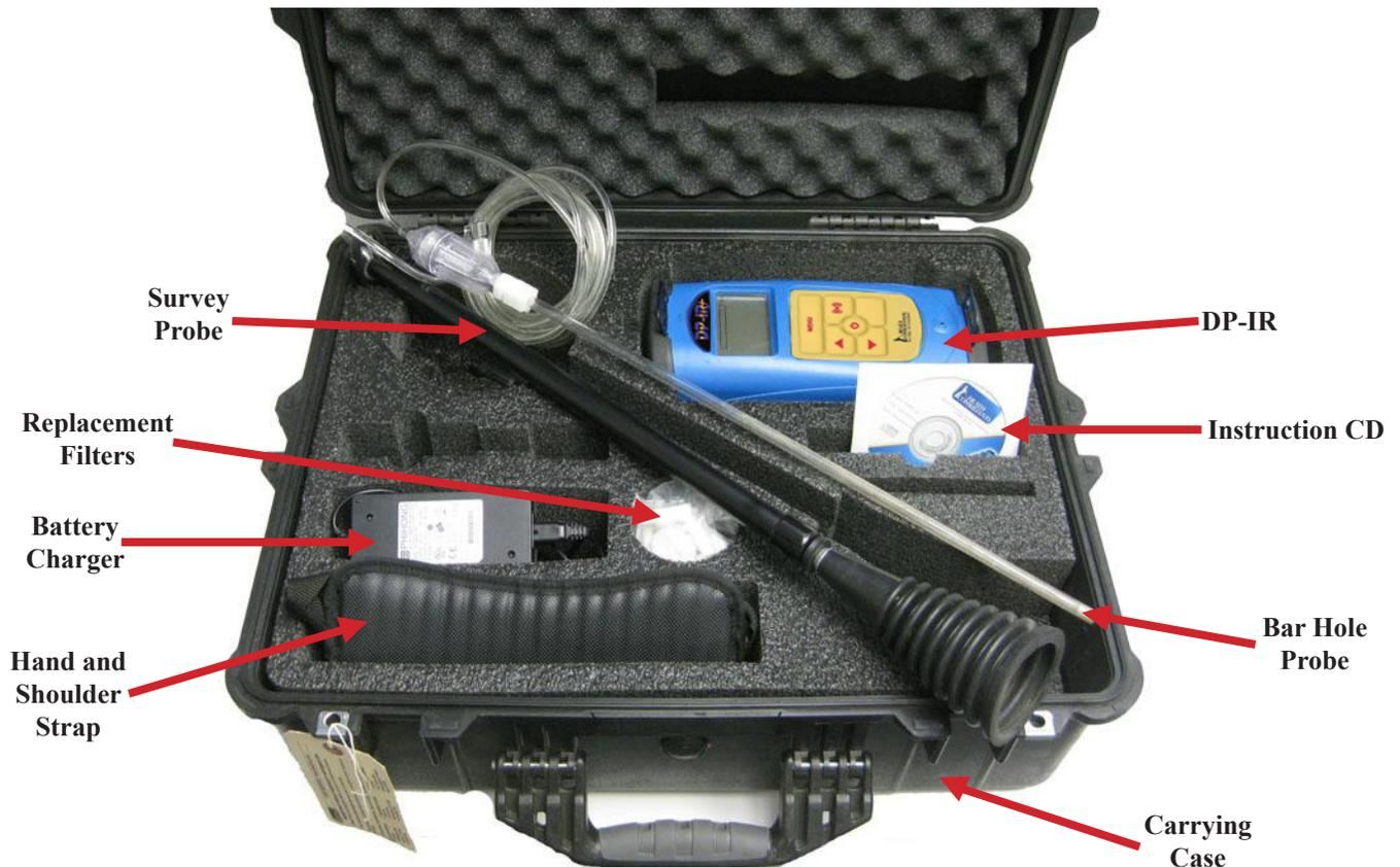
**Figure 2: System Components**
