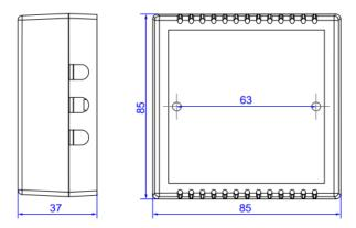
3. Use rounded cutouts on the side of the base to let in the cables from the power supply and of the external devices as shown below.
