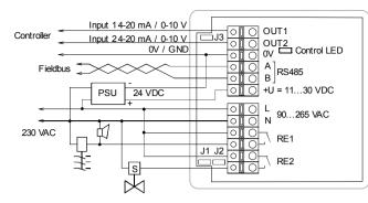
To power the instrument from an external 24 VDC source, connect terminals 0 V and +U to the source. If an integrated mains power supply module is used, connect terminals L and N to the mains.
