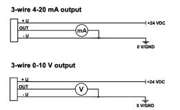
The terminals on the E2615 series devices are suitable for a wide range of wires with a cross-section of  $0.2...1.5 \text{ mm}^2$ . We recommend to strip the wire end by 8...9 mm and use wire end sleeves.
