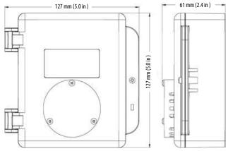
Above dimensions are shown with optional splash guard. Without splash guard, thickness is 53.34 mm (2.1 in). The area required for enclosure door to be open 90 degrees is 178 mm (7 in) or 254 mm (10 in) for fully open. With the splash guard, the enclosure has an IP54 rating.
