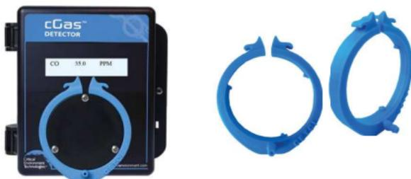
**NOTE:** The Cal Clip is designed to prevent entry or exit of air except via the hose barb fitting, therefore it **must be removed during normal operation** or else the gas readings will not be accurate.
