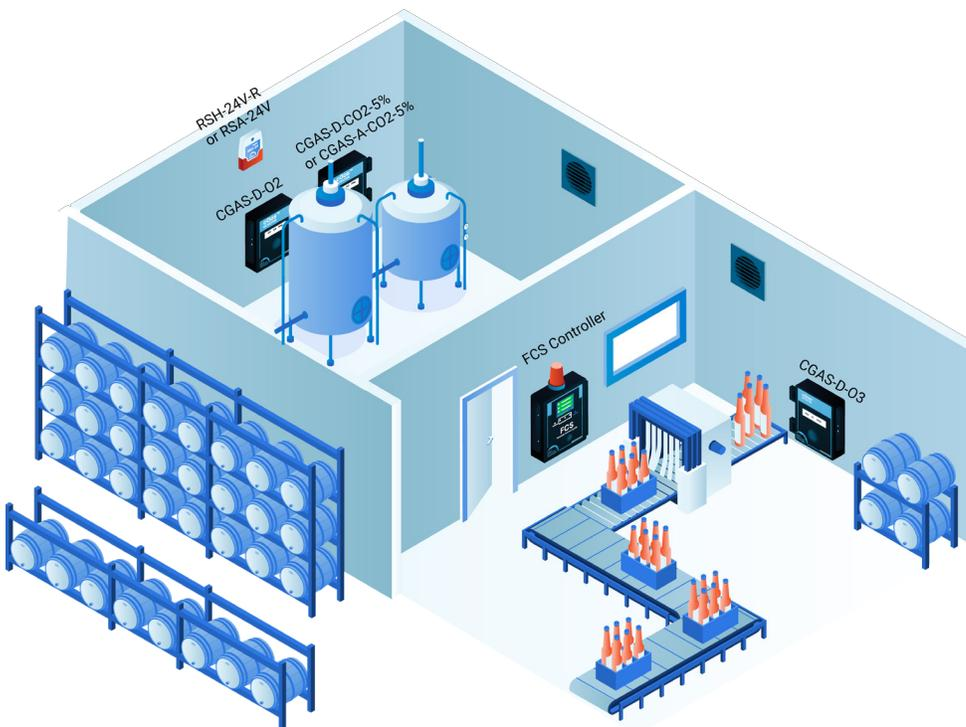
mounted on the wall near the CO<sub>2</sub> detector at the breathing zone height. It should be close to the fermentation tanks where oxygen is most likely to be depleted in the event of a build-up of CO<sub>2</sub>. The measurement range for O<sub>2</sub> is 0 - 25% volume. With the optional splash guard installed, both enclosures are water tight (IP54 rated) and will withstand water spray or wash down applications.
