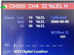
The details screen allows you to view the alarm level setpoints, priorities it is assigned to, the type of fault, when it was last calibrated, its Modbus® ID, and a description of the location of the transmitter for that particular channel.
