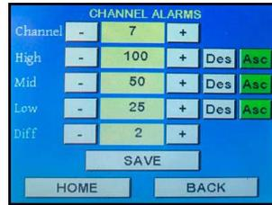
If you want to review the current settings for each channel, press the + or - button to scroll through the summary screen of each channel or use the keypad to enter the specific channel number.
