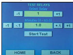
Enter the relay number you want to test and enter the length of time you want to test the relay for. Press Start Test to begin the test.
