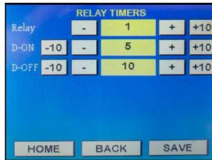
If you want to review the current settings relay by relay, press the Relay + or - buttons. To skip ahead by 10 sequential relays at a time, press the +10 button. Or press the yellow field to reveal the keypad to enter a specific number.
