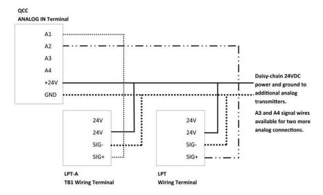
**NOTE:** DO NOT use solid-core wire for connection to wiring terminal strip. Any damage caused by using solid-core wire will void warranty. Use stranded wire ONLY. Under most local electrical codes, low voltage wires cannot be run within the same conduit as line voltage wires.
