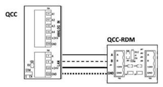
Either TB2 or TB3 can be used to connect the QCC to the QCC-RDM. Both are Modbus® connections. The QCC-RDM will automatically broadcast the display information to Modbus® ID 253. This is the common
