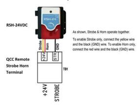
Multiple horn/strobe devices can be accommodated by using the relays. A remote power supply may be required.
