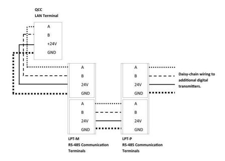
**NOTE:** DO NOT use solid-core wire for connection to wiring terminal strip. Any damage caused by using solid-core wire will void warranty. Use stranded wire ONLY.
