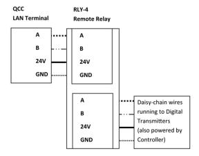
**Note:** This diagram shows the RLY-4 connected directly to the QCC, followed by digital transmitters connected in a daisy-chain fashion. The RLY-4 could be connected anywhere along the digital network in a daisy-chain fashion as necessary.
