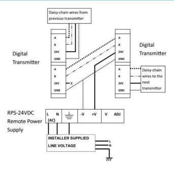
**NOTE:** Observe polarity when connecting DC load to the output of the power supply.
