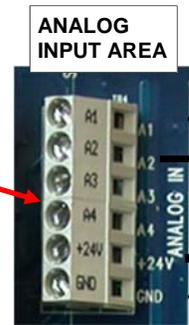
A1 TO A4 ARE INDIVIDUAL 4-20 mA SIGNAL WIRE CONNECTIONS FOR EACH AST-IS18
