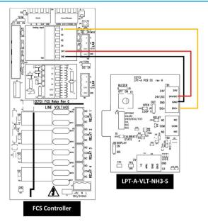
When connecting analog transmitters, the 24 VDC power supply and GND can be daisy-chained to the next transmitter. Each signal wire is connected directly from the Controller to each transmitter.
