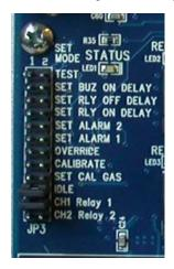
To start a configuration, place one jumper on the channel / relay selct position CH1 Relay1 and place the other jumper on the function position you want to configure:
