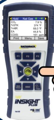
The Bacharach Reporting App is a user-friendly, feature-rich method for getting your combustion data into the "real world." Simply transfer the data from a combustion analyzer to your mobile device, then view, save and email the data – all at the touch of a button. Up to 100 records can be saved to your mobile device. Any of these records can be used to generate a custom as-found/as-left report, which can include technician/company information, company logo and customer information.
