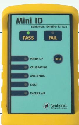
Easy to use with 'PASS' or 'FAIL' result indication for system under test
