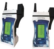
The YESAIR is available with an externally mounted particulate sensor for monitoring particulates in the air. The particulate sensor detects smoke, dust, pollen, spores, etc. particle concentrations in air by using an optical sensing method. A laser LED and a photosensor are optically arranged in the device and the photosensor detects the laser LED light reflected by dust particles in air.
