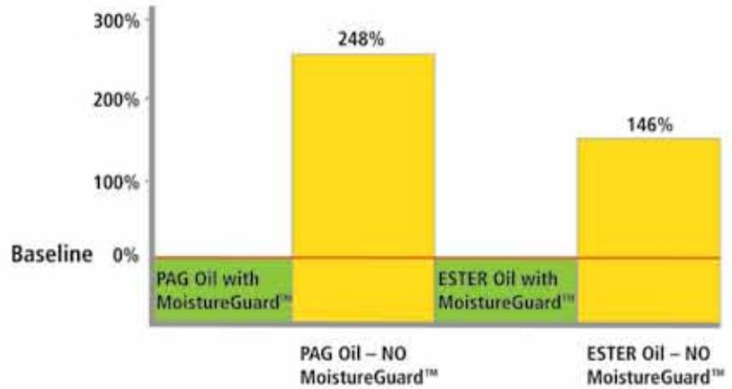
*Test simulates the shelf life of a sealed container of A/C Oil. The test was conducted in an environmental chamber using sealed containers. (This represents a two year shelf life)*
