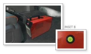
Ensure the machine is level. Center air bubble. (Inset Photo B) Start the vehicle. Vehicle must be running for the duration of the treatment.
