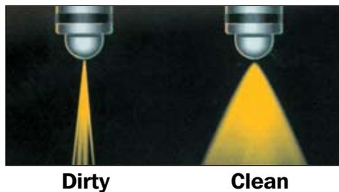
The above diagram shows that dirty injectors impede flow and dispersion of fuel while clean injectors improve fuel system efficiency and performance.
