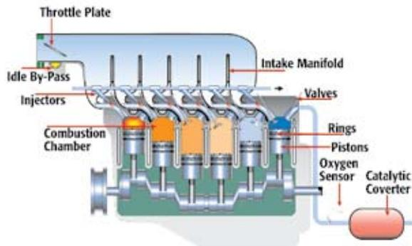
The cleaning process starts from the air intake, throttle body, injectors and fuel rail to the combustion chambers, valves, oxygen sensor and catalytic converter.
