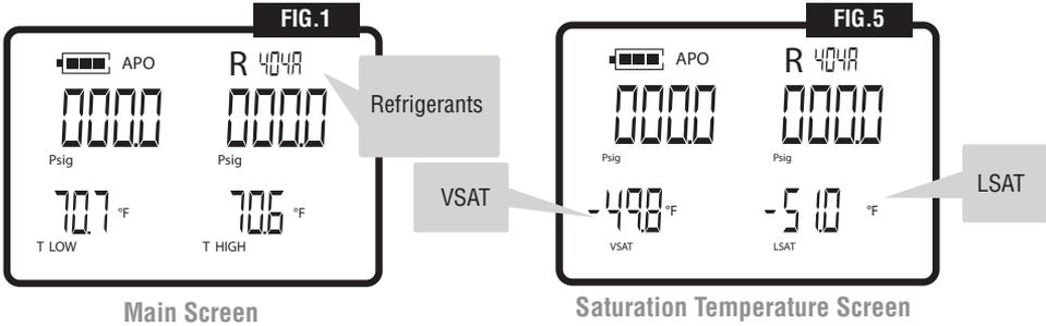
3. Note: In this mode, and to prevent errors, refrigerant cannot be changed using **[REF]** key. Press **[CLR]** to return to the **Main Screen [FIG.1]** from this view.
