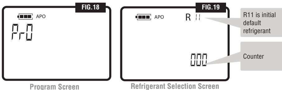
3. The **Initial Refrigerant** (blinking in upper right) should be R-11 and Counter (Lower Right) should start at 000.
