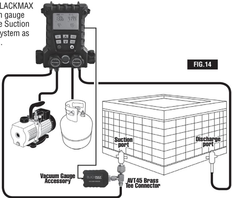
4. In this mode, the manifold will show current vacuum in the system. The display begins to show vacuum levels at 25000 microns or less and is accurate to +/- 10 microns. Continue to run vacuum pump until the desired vacuum level is reached. Once reached, proceed to Vacuum Hold Test.
