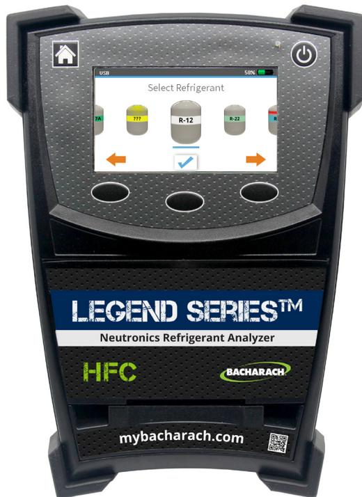
Clean air calibration is all you need to analyze your refrigerant in less than 2 minutes. No matter the application, Bacharach's Legend HFC Refrigerant Analyzer is capable of measuring vapor or liquid refrigerant to confirm purity while detecting the presence of other harmful refrigerants or air.
