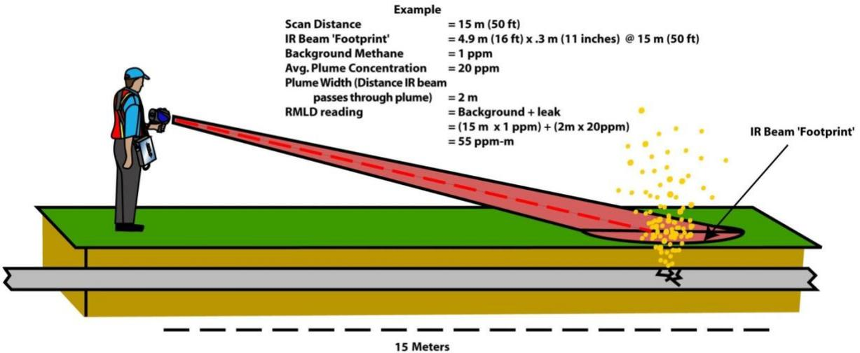
**Fig. 4-5: The ppm-m reading is the product of the plume concentration times the distance the IR beam passes through the plume (plume width) in addition to any background gas. As the scan distance increases, the size of the infrared beam “footprint” increases.**
