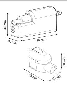
Hose diameter Suction : 4/6 mm - supplied Discharge : 6/9 mm - not supplied
