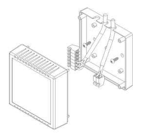
For easier connection, terminal blocks of E2610 series devices are removable. To dismount the terminal block, pull it off from the PCB. Connect the power terminals N and L to the 24 V power source if you are using detector version -24 or to 230 V AC mains if you are using detector version -230 (see diagram below).
