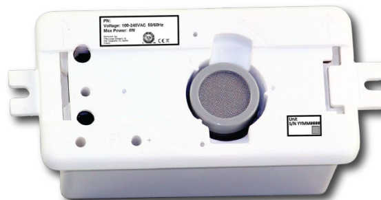
Figure 22. UK Version of MVR-300 and Representative UK Back Box
