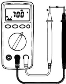
▫ Connect the red test lead to the anode side and black test lead to the cathode side of the diode being tested.
