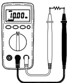
⇒ Connect red test lead to "  $\Omega$  "jack and black test lead to " COM "jack.
