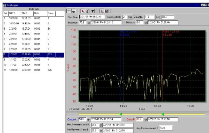
When you have Sound Level DATA LOGGER meter connected to PC and select "DataLogger" from main menu or click
